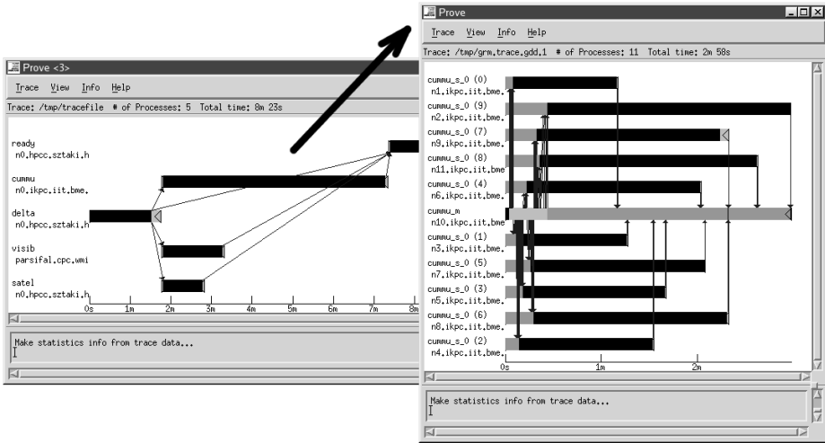
Fig. 2. Space-time diagram of the whole workflow and one of its component jobs
